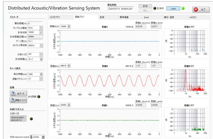
Vibration distribution display example (left: 3D vibration waveform, right: 2D vibration waveform)
